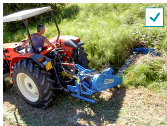
↑ FIGURE 4.2.11 An example of good practice: mowing with a sickle bar mower, thus ensuring the appropriate cutting height (Source: Brilliant Ltd., website 2021)
