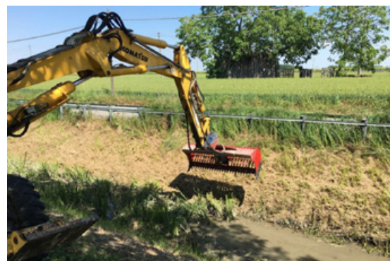
An example of mechanical equipment for mowing the banks and slopes with a sickle bar attachment (Source: Wasserverbandstag 2015)
