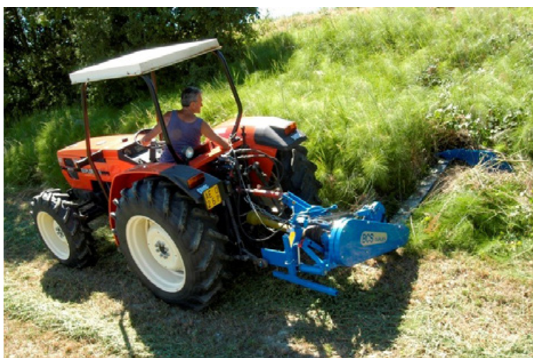
An example of mechanical equipment with a sickle bar attachment used for mowing floodplains and embankments (Source: Brilliant Ltd., website 2021)
