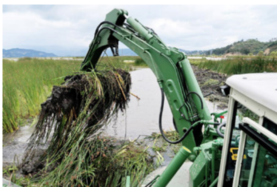
A floating dredger removing macrophyte vegetation and silt from a watercourse bed (Source. Aquamec Ltd., website 2021)
