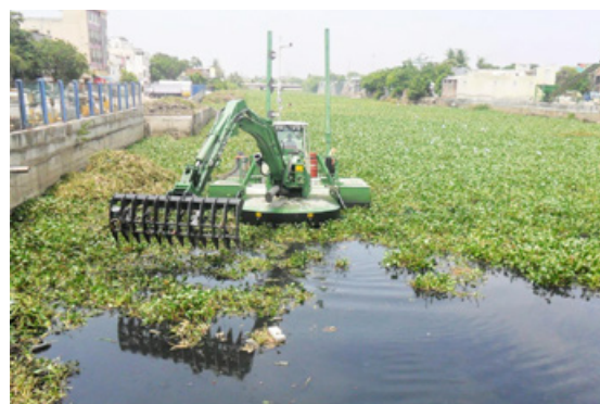
Removing macrophyte vegetation from a watercourse bed with a floating dredger (Source. Aquamec Ltd., website 2021)
