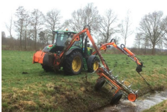
An example of mechanical equipment for mowing aquatic macrophyte vegetation on the banks (slopes) with a sickle bar attachment (Source: Wasserverbandstag 2015)
