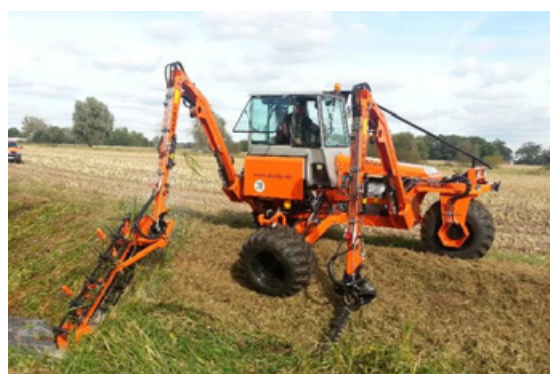
An example of mechanical equipment for mowing the banks and slopes with a sickle bar attachment (Source: Berky Company, website 2021)
