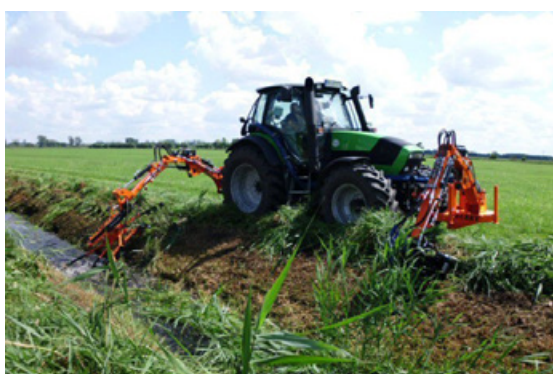
An example of mechanical equipment for mowing aquatic macrophyte vegetation in the bed and on the banks (slopes) of a watercourse with a sickle bar attachment, without a grab basket (Source: Wasserverbandstag 2015)
