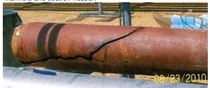
Figure 2. Ruptured 12-inch diameter end cap of low-temperature suction line piping on the roof of the facility.
