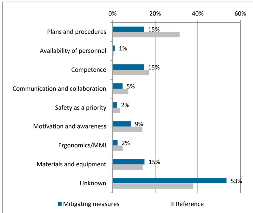
Figure A3.16. Why did the mitigating measures fail – percentage of cases in which elements are relevant to the mitigating safety measures.
