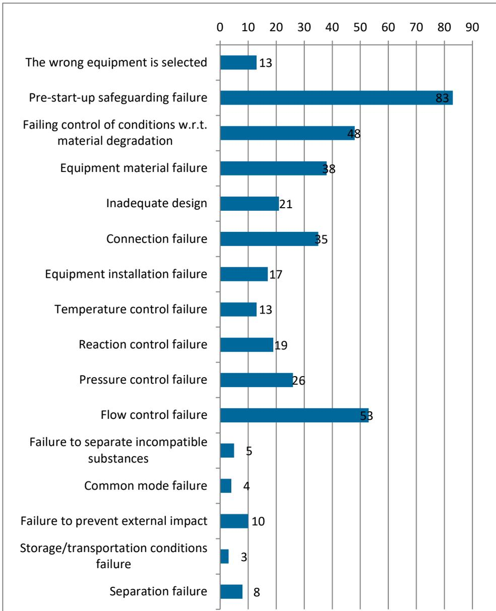
Figure A3.4. Safety measures in the 1<sup>st</sup> LoD – number of times the safety measure failed.
