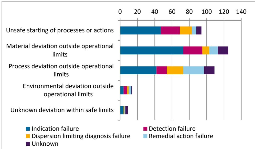
Figure A3.8. Ways in which recoveries failed.
