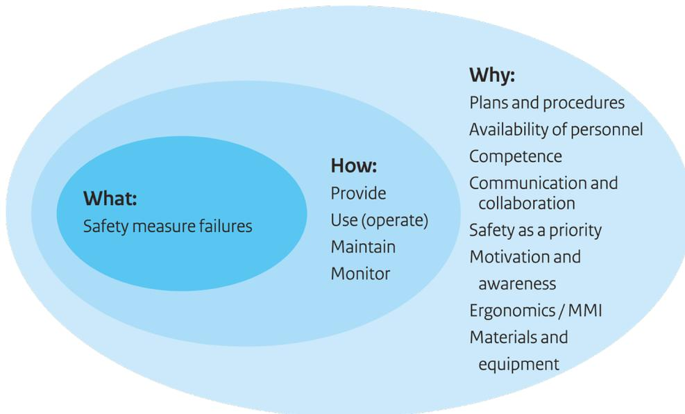
Figure A1.2. Structure for the underlying factors in the analysis model. The MDS management delivery system failures (why) precede the task failure (how), which precedes the barrier failure (what).
