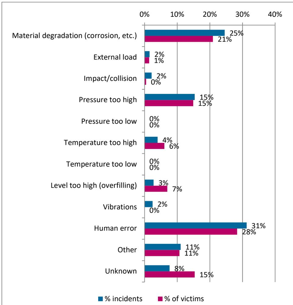
Figure 2.9. Immediate causes of the accident.
