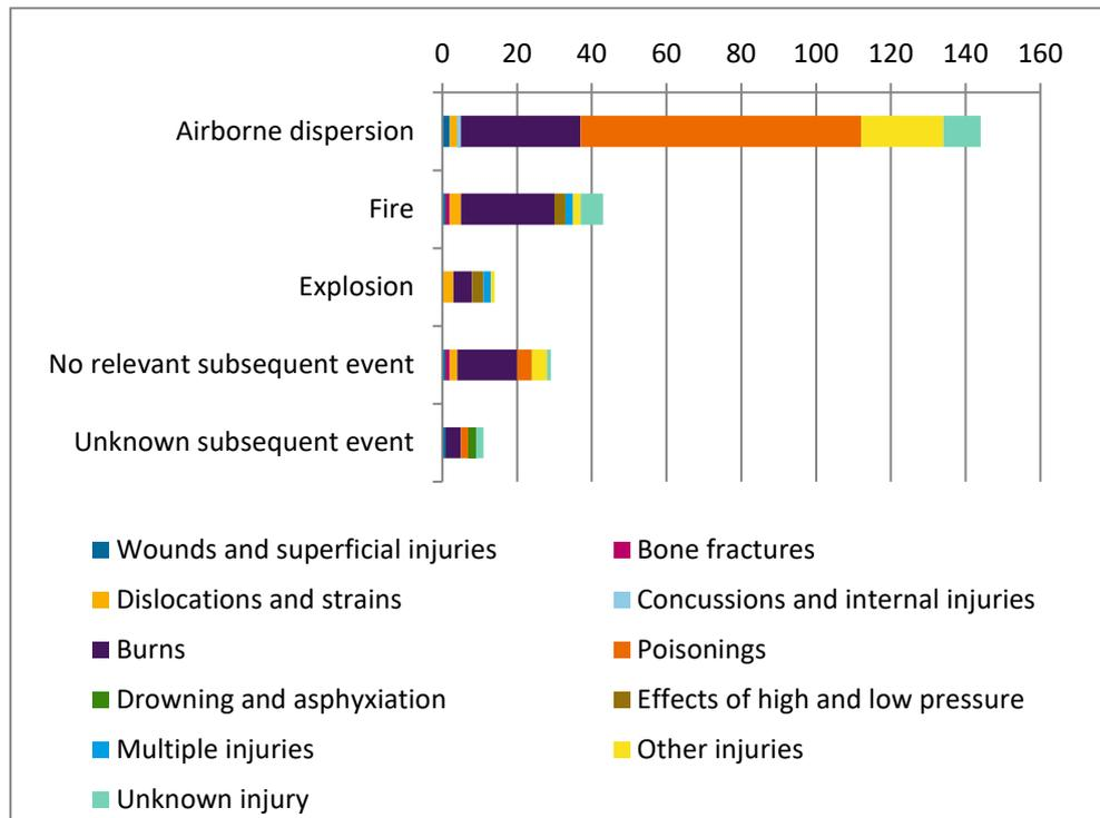
Figure A2.2. Type of injury in combination with type of subsequent effect (number of victims).
