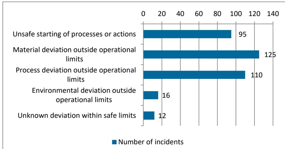
Figure 3.4. Deviations outside the operating window.
