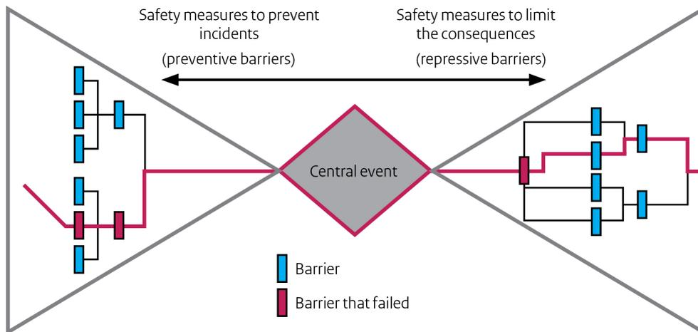
Figure A1.1. Storybuilder model with the incident path represented as a red line. This indicates the route of the incident scenario that occurred and the associated barrier failures.
