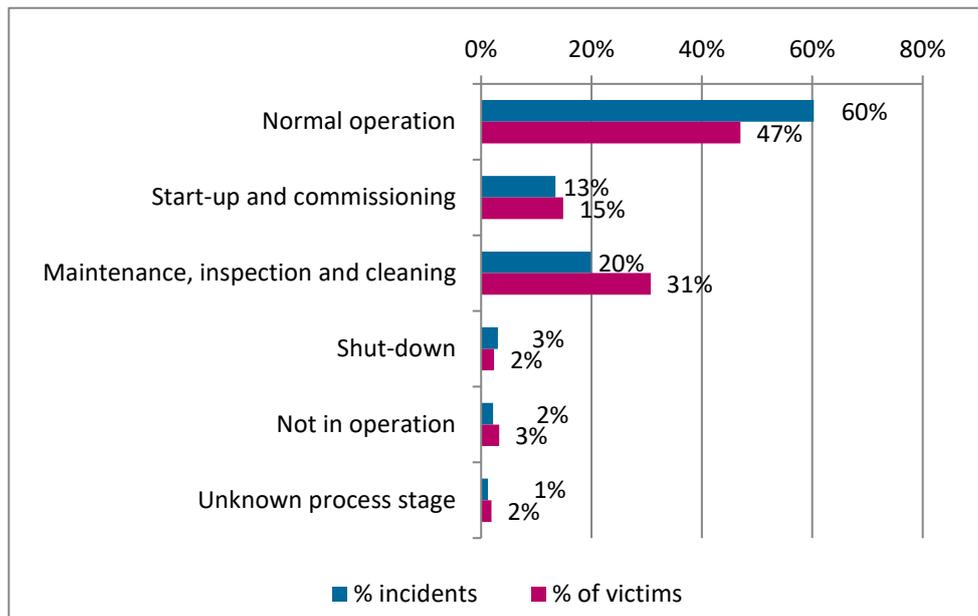
Figure 2.8. Process stage prior to the accident (percentages of total).
