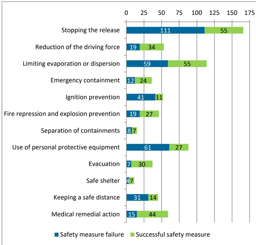
Figure 3.8. Mitigating safety measures: number of times these measures failed or were successful.
