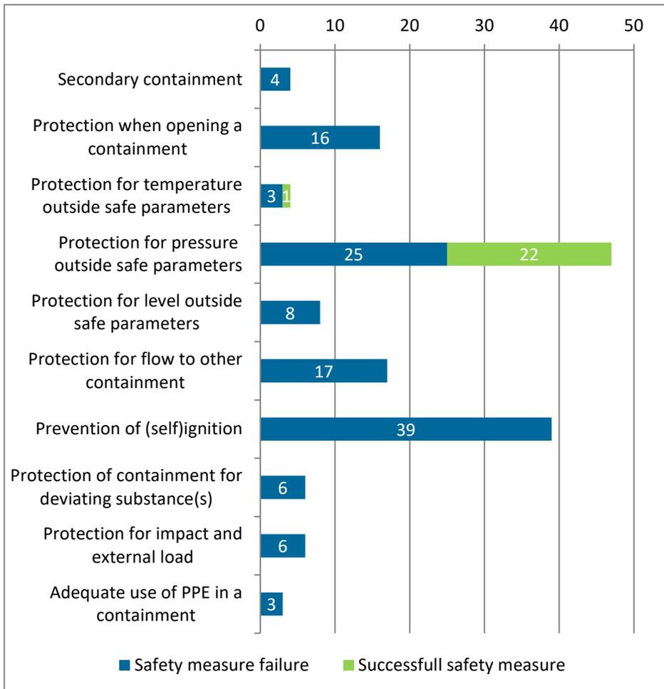
Figure 3.7. Safety measures with regard to emergency protection: number of times that the safety measure failed or succeeded. Note: the 3<sup>rd</sup> LoD was only relevant for 41% of all incidents.
