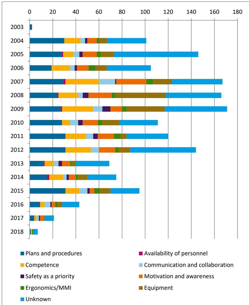
Figure 5.3. Underlying causes of safety measure failures (number of Management Delivery System failures).
