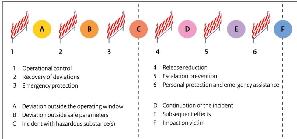
Figure A1.3. Summary of the Storybuilder MHC model. The lines of defence are represented by fences, the loss of control events by circles. The central event (C) is in the centre.
