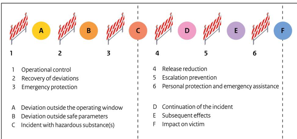
Figure 3.1. Lines of defence (represented by numbers) and the consequences of any failure (represented by letters) in the analysis model.
