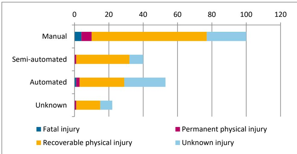
Figure 5.8. Method of task or process automation and severity of injury.
