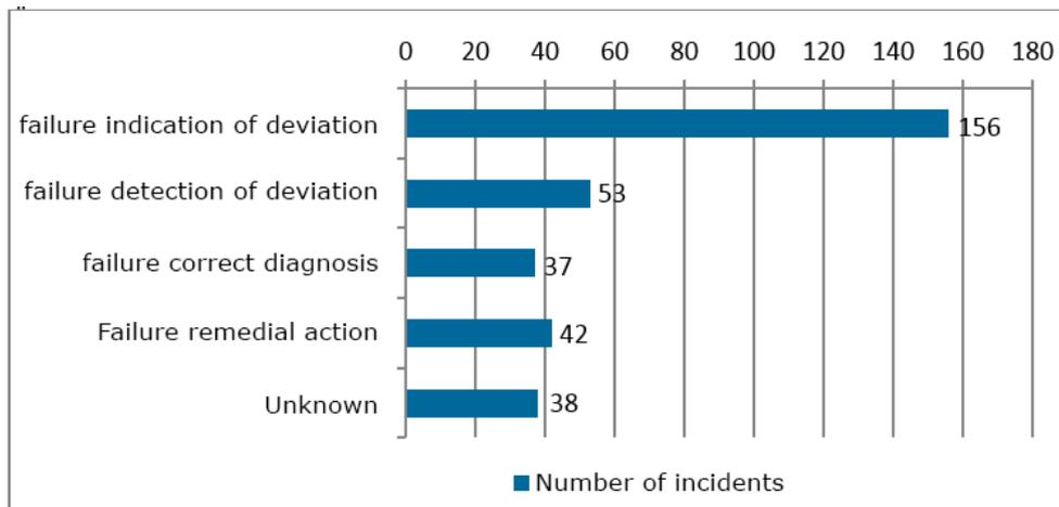
Figure 3.5. Ways in which recovery of deviations fails.
