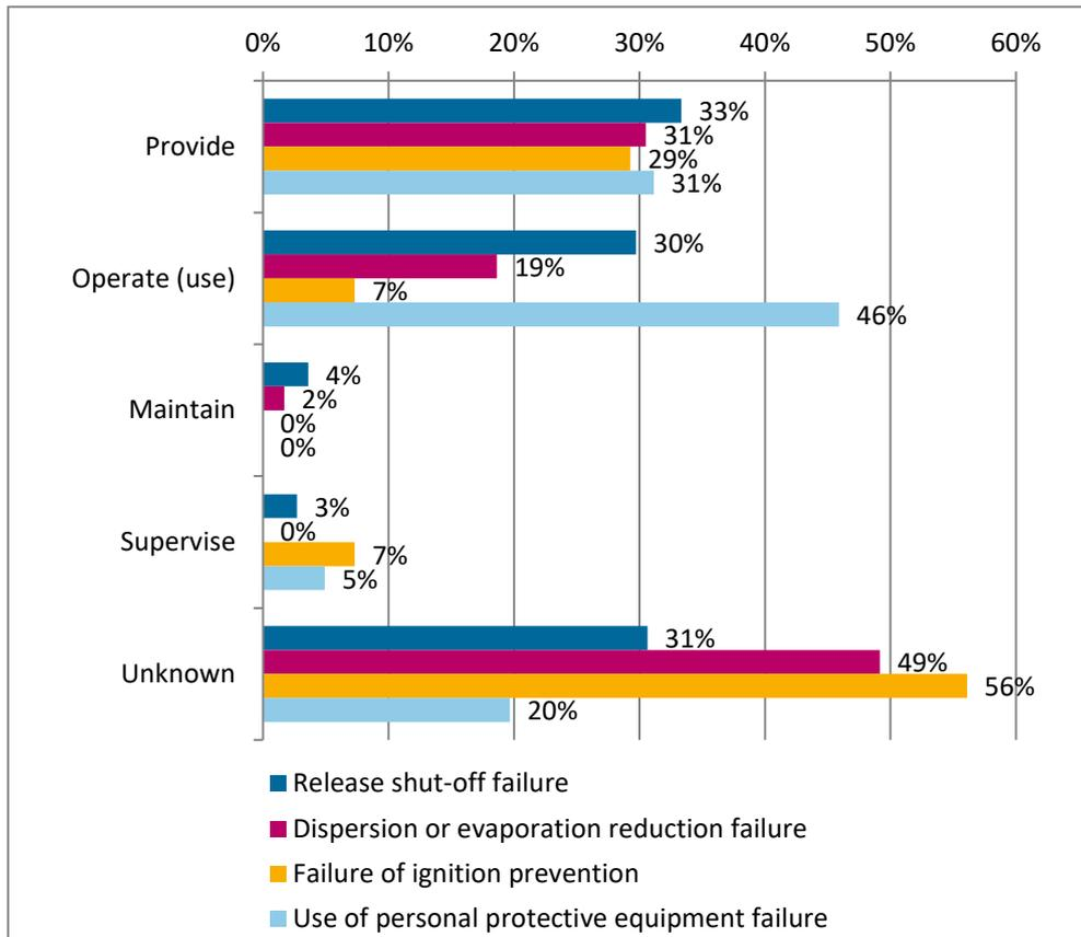
Figure A3.15. How did the mitigating measures fail? Selection of the four mitigating measures that fail most often.
