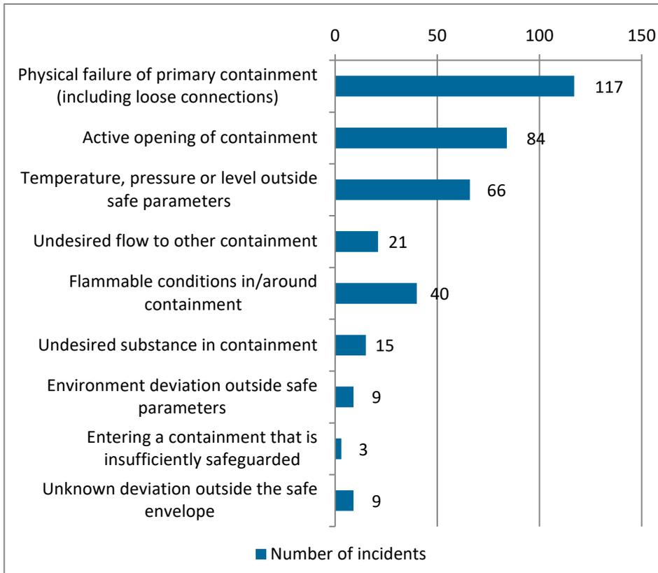
Figure 3.6. Deviations outside safe parameters.
