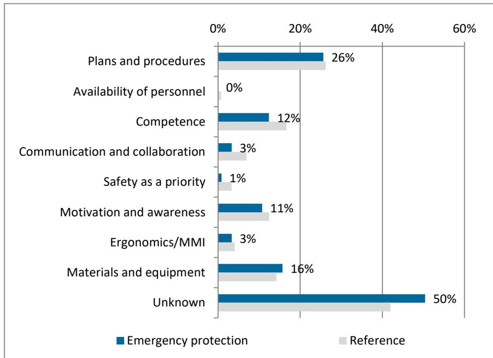
Figure A3.13. Why did the emergency protection fail – percentage of cases in which elements are relevant within the 3<sup>rd</sup> LoD.
