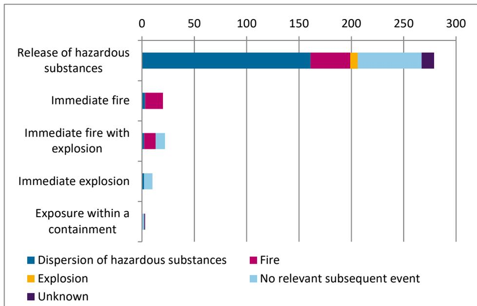
Figure 2.3. Type of incident: immediate effect and subsequent event<sup>9</sup> (number of incidents).
