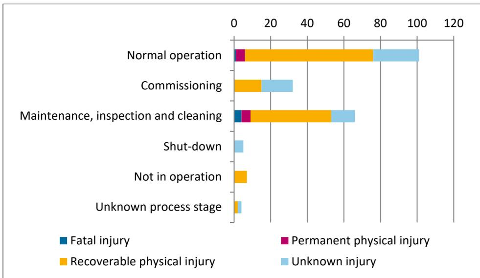
Figure 5.7. Process stage and severity of injury.
