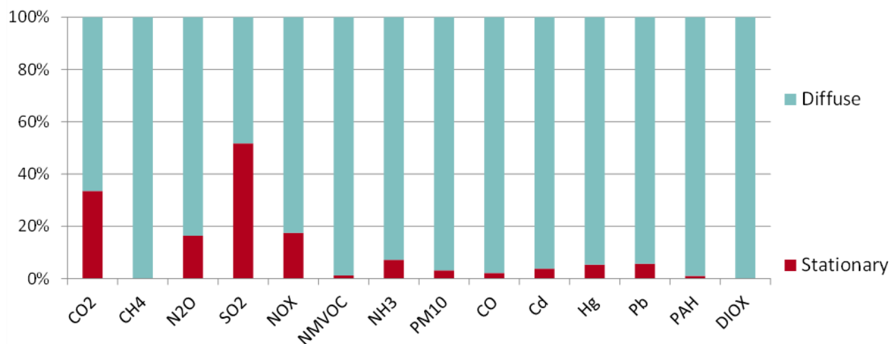
Figure: Split of E-PRTR point sources (“stationary”) and diffuse emissions for various pollutants (for Croatia, 2014)
